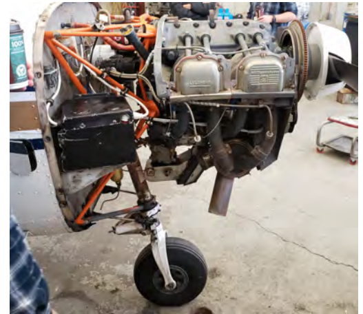
A look at the engine off PFC's Cessna 152, GZSA, undergoing its 100-hour inspection. (Photo: Phillip Souder)
