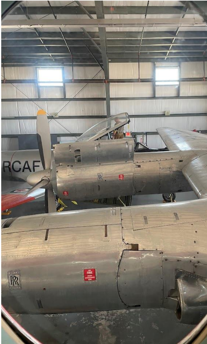
(Above: Cowlings cover the Rolls-Royce Dart turboprop engines of BCAM's Vickers Viscount, seen from inside the cabin through the Viscount's large oval windows. Photo: Florian Krauthan)
